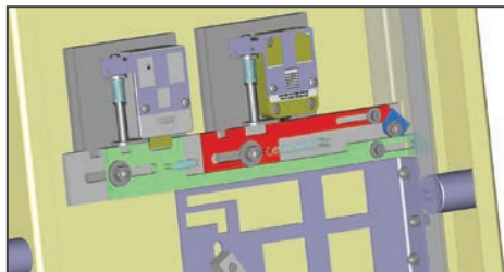
Safe open – Lock on the right unlocked, lock on the left locked, bolts retracted
