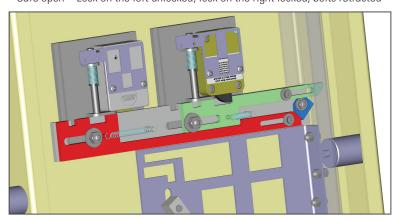
The redundant boltwork means the two installed locks operate completely independently. Unlocking either lock allows access to the safe. This design gives safe owners the protection of redundant locks to protect against any type of lock failure.
